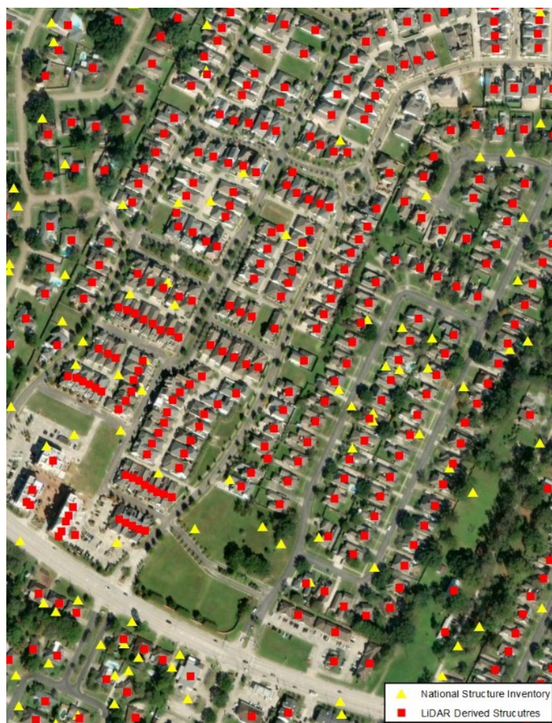
Figure 71: Comparison of LiDAR derived structures (red squares) and the NSI (yellow triangles) in East Baton Rouge parish.
