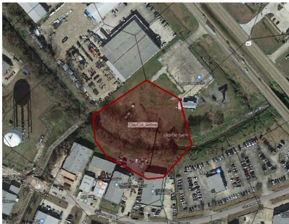
Figure H-15 2D Boundary Condition Line for Flow into Claycut Bayou near Airline Highway
