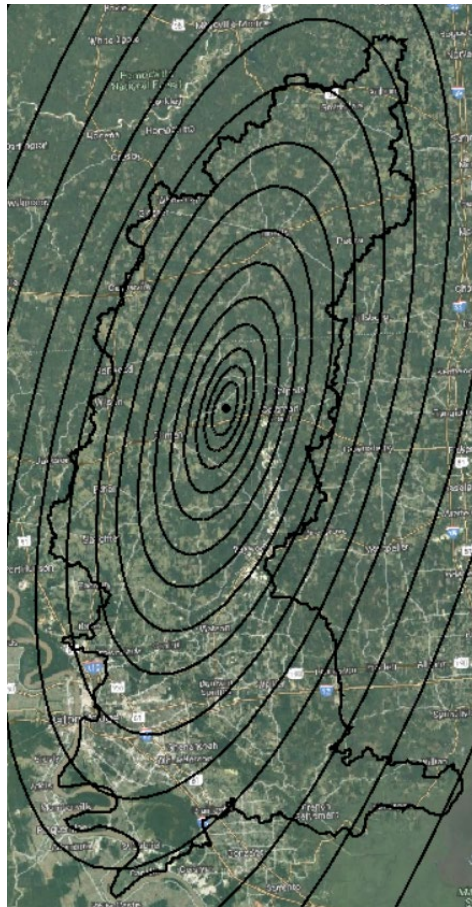
Figure H-3 Design Storm Location and Isohyets
