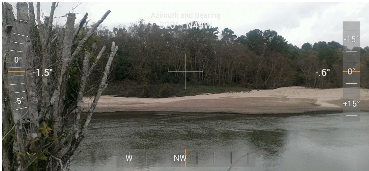
Figure 26: Amite River, Cross section 399176.7 (approximately 20 miles upstream of the Comite River Confluence), looking at right over bank. The basic right overbank Mannings's N value is estimated to be 0.12. Photo: Forte & Tablada, 2018
