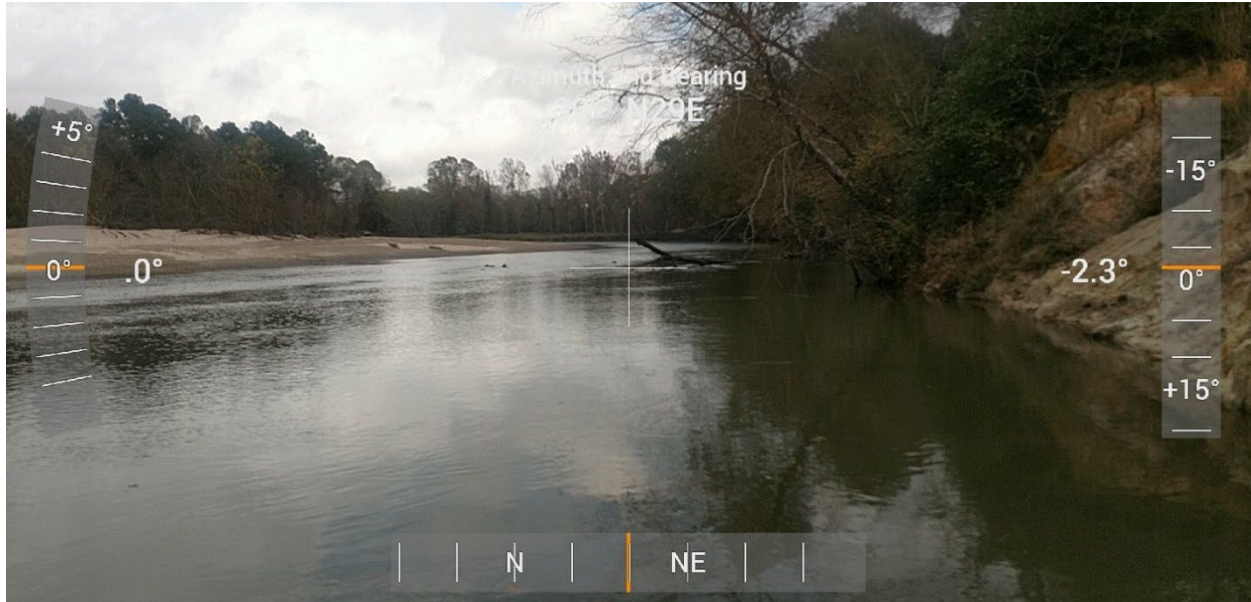
Figure 25: Amite River, Cross Section 399176.7 (approximately 20 miles upstream of the Comite River Confluence), looking upstream. The basic channel Manning's N value is estimated to be 0.037.
